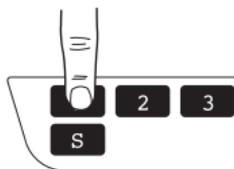
**NOTE:** The readout will show, for example, S (number) until the double click is heard and then the height readout will return.
