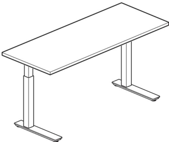
**NOTE:** Avoid risk of injury with your height-adjustable table through proper training. For safe operation, ensure that there is at least 1" between the height-adjustable worksurface and any adjacent objects such as storage or fixed worksurfaces.
