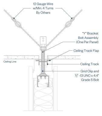
Base building construction must be in accordance to local site building code requirements
