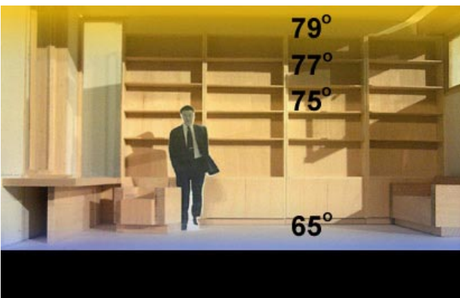
Air Temperature Stratification
