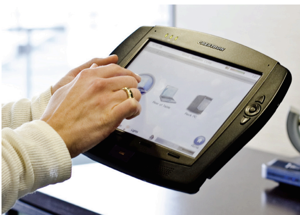
Crestron handheld devices are used to control audio and video equipment.
