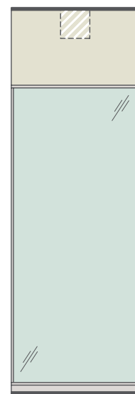
COMBINATION GLASS-SOLID TOP CUTTABLE
