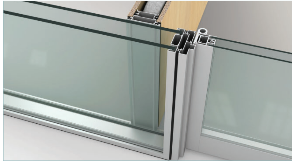
FLUSH FLY-BY, EFG 2 CHANNEL
